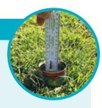
With this information, you can plan how long you should water each week and check water is applied uniformly. If the cans don't fill up evenly, individual sprinkler nozzles might need adjustment.
