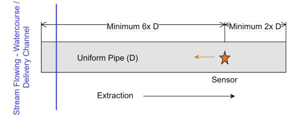
For all other installation scenarios, the velocity sensor must be installed with the upstream and downstream lengths specified in the Meter Installation Plans in Appendix D – as a minimum.
