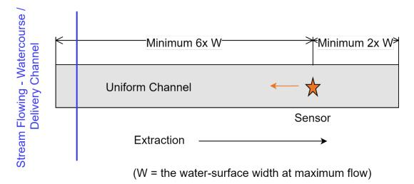
Where there is upstream disturbance (i.e., high velocity flow via a sharp bend/there is an angled sluice gate) upstream, the velocity sensor must be installed to these minimum straight length requirements.
